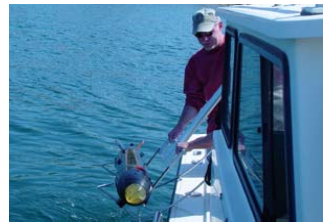
EdgeTech 2200-S installed on an AUV
