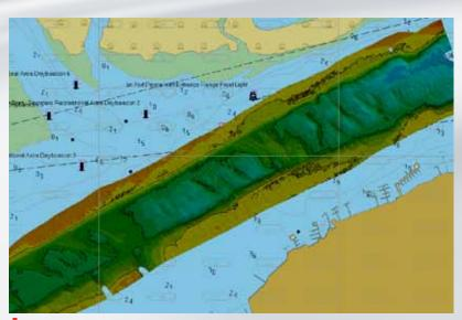
EdgeTech's 4600 is a combined, fully integrated, swath bathymetry and side scan sonar system. The 4600 produces real-time high resolution three dimensional (3D) maps of the seafloor while providing co-registered simultaneous side scan and bathymetric data.
