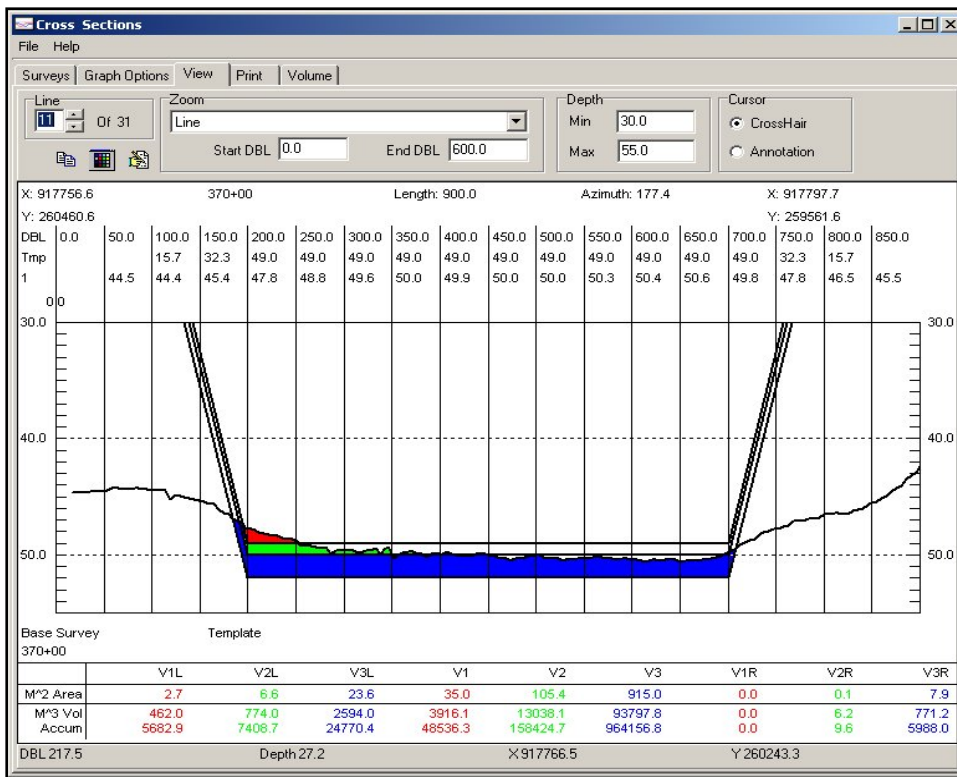
A display of a sectional profile showing the depth profile and the design template in the CROSS SECTIONS AND VOLUMES program. [Data courtesy USACE Buffalo]
