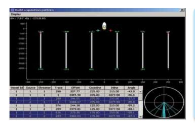
SeaPro Bin is a binning tool that manages several 3D seismic marine surveys for different users in a professional environment. SeaPro Bin provides flexible tools to interactively manage the seismic surveys from 3D through to WAZ.
